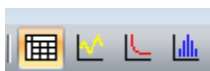
Fig 6 Data viewing buttons in top left. From left to right: grid: datalog grid, yellow line: datalog graph, red line: correlation graph, blue lines: regularization graph.
