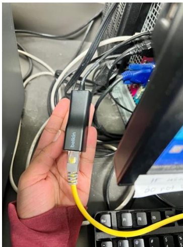
Fig 2 Unplug yellow cord to connect your laptop with the instrument.
