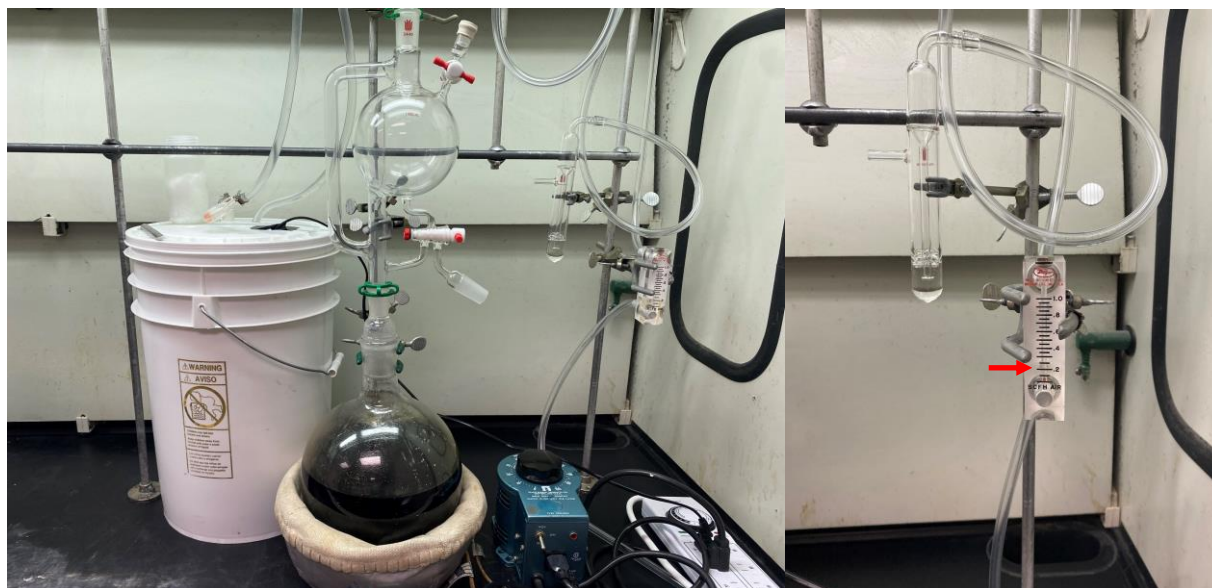
Figure 4: Left – The fully assembled THF still ready for operation. Right – The flow meter with a red arrow showing the correct flow rate.
