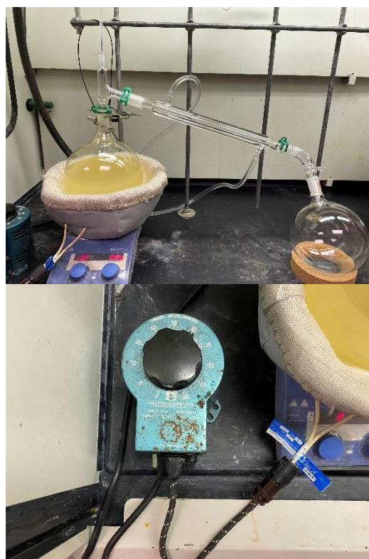
Figure 2: Top – Set up for distilling THF. Bottom – Set up for Variac (set to 60).
