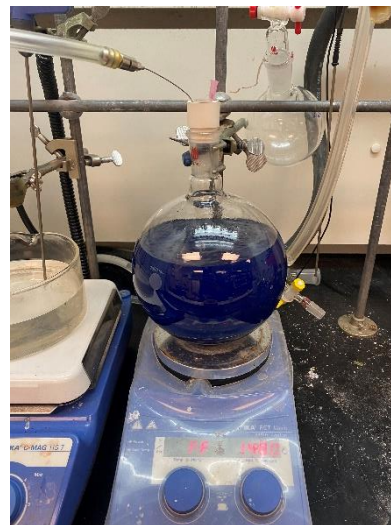
Figure 3: THF/sodium mixture after the addition of benzophenone and degassing with nitrogen.
